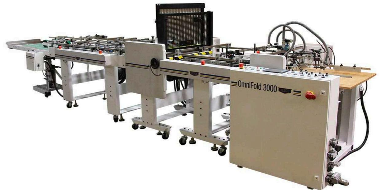
Kluge **OmniFold** 3000 Automatic Folding and Gluing System
